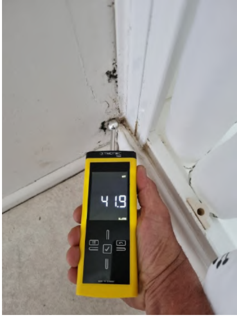
Water ingress visible in the past with the shower
