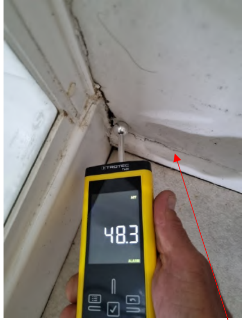
Water ingress visible in the past with the shower
