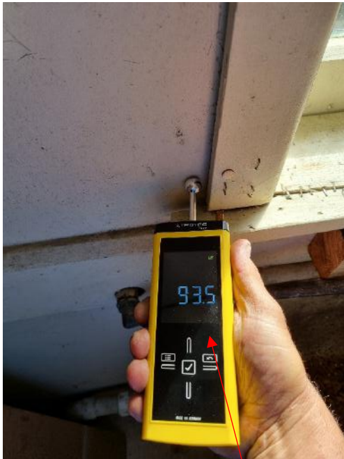
Moisture meter reading is greater than 80, this means material is at risk for wetness – further investigation is required
