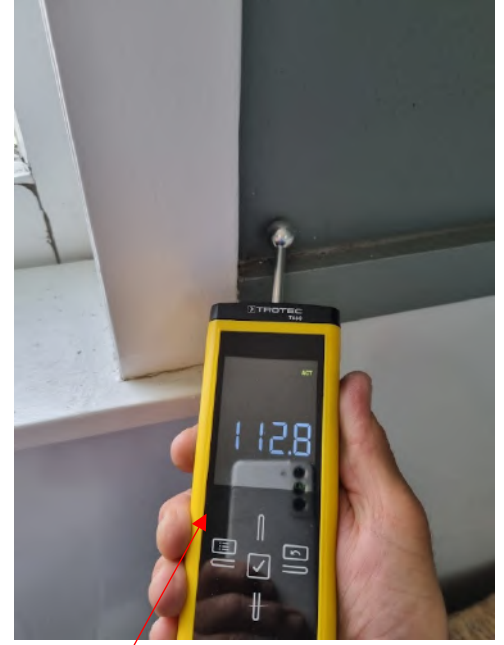
Moisture meter reading is higher than 80, this indicates great risk for wet material and further investigation is required
