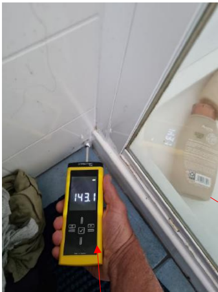
Moisture meter readings are higher than 80, this indicates there is wet materials and is at risk. Further investigation is required
